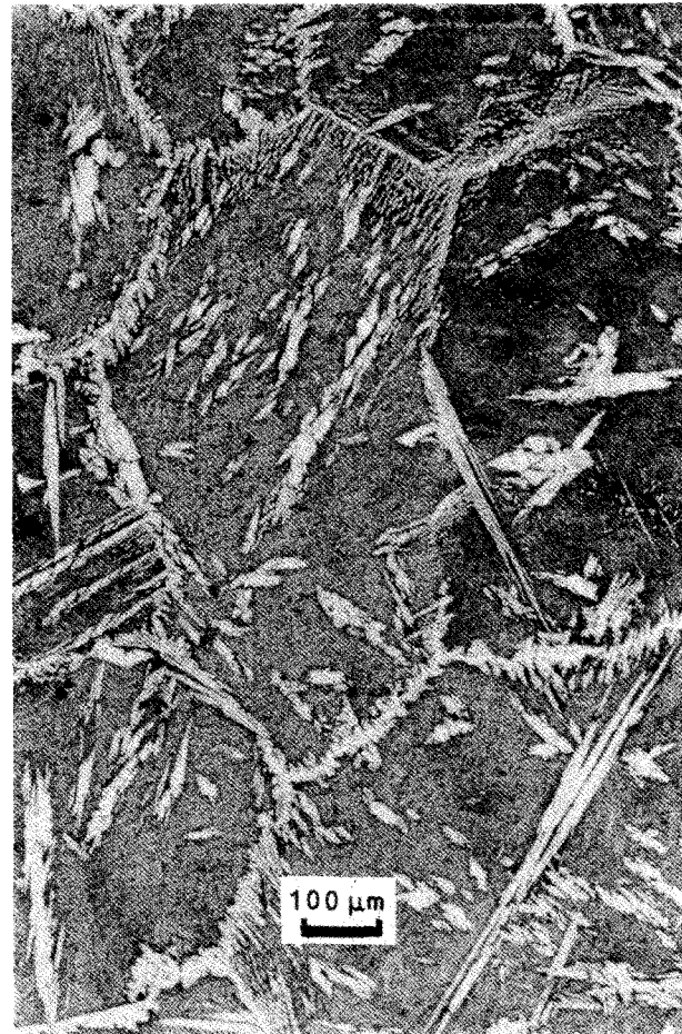
Figure 19 Microstructure of alloy M1902 in Beraha's No. 1 tint-etch solution. Austenite light, ferrite dark.
